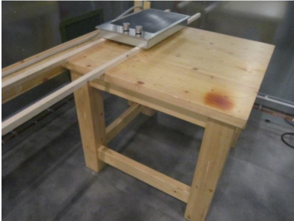
DISTURBANCE POWER SETUP
