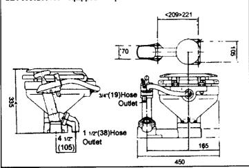
Fitting details: Connections for 19 mm. W4") inlet hose and 38 mm. (1 112") outlet hose
