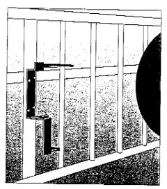
1. Mount the bracket on the vessel using four M8 or 5/16 inch bolts.
