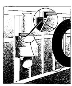
**4.** Attach the signal to the life buoy with a line of minimum 4 m length and 8 mm diameter. Use a bowline hitch and ensure that the line goes all the way around the signal.
