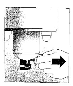
**5.** Remove the transport safety pin. (Keep the safety pin for future use.)
