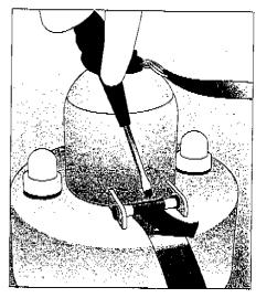
2. Use a sharp object to remove the plastic tube from the MOB. On the MOB Light & Smoke, the two lights should then light up.
