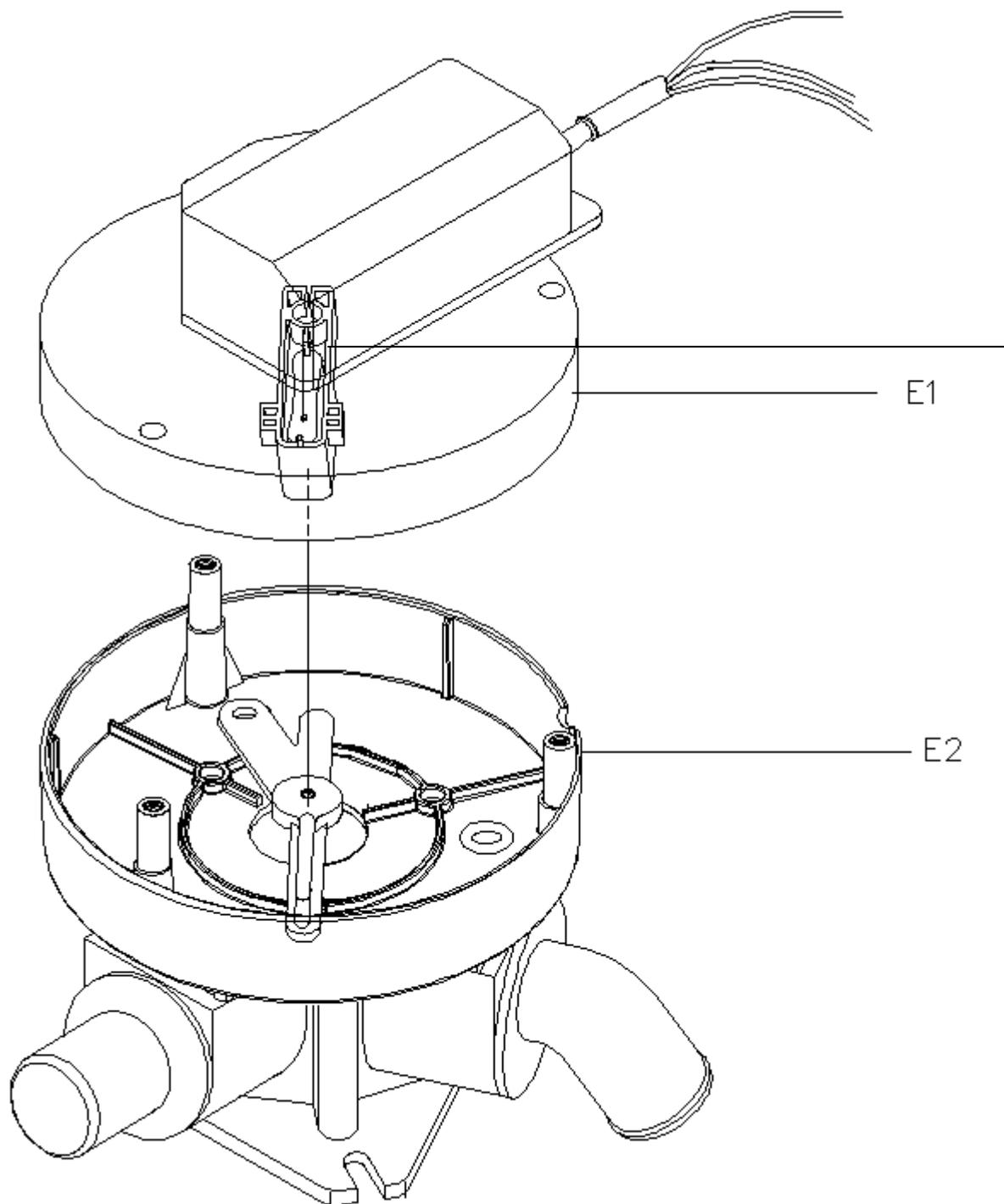
Step 5. Finally assemble E1 and E2 together with Screws A1(M4X18).
